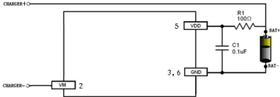
**Fig 6 XB5306A in a Typical Battery Protection Circuit**
